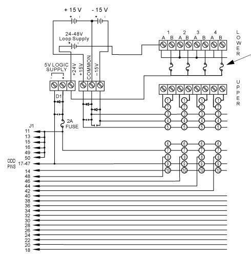
Install 1/8 amp fuse here to use the 24 VDC shared loop source. With fuse installed, shared loop source + 24 VDC is available at lower B terminal. Fuses are provided with AD3, DA3, and DA8 modules.
