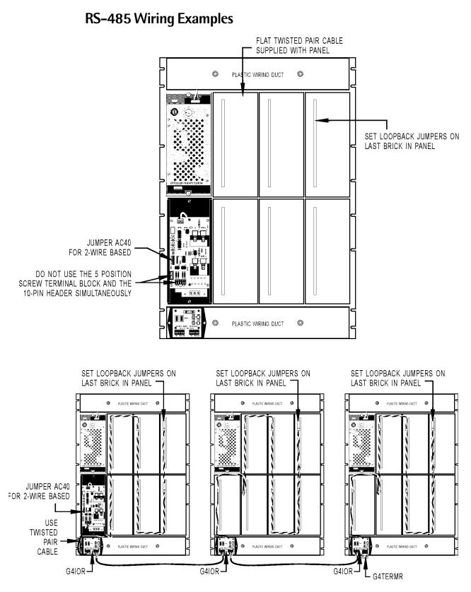
NOTE: When only one panel of remote bricks is attached to the AC40, use the 10-pin header.
