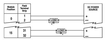
\*Note: Commutation diode must be used on inductive loads. Typically, use diode 1N4005
