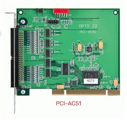
The card includes a 50-pin male header connector and is compatible with HH-series and OD-series flat-ribbon cable. Four LEDs on the card indicate card operation.
