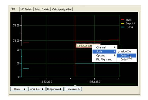
**17.** To measure the system lag (the time between the change in output and the change in input), click and drag the first vertical red bar to just after the output change. Drag the second bar to just before the change in input.
