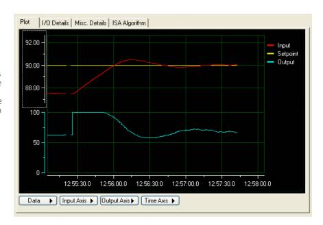
**10.** If derivative correction is needed, experiment with the derivative constant: in the Tune D field, type 1 and click Apply. (Your PID loop may require a larger number.)
