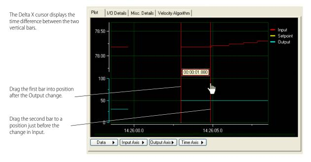
If you are unable to get the precision you want, you can view the plot at a lower time span, such as 10 seconds. You will need to reposition your plot and the measurement bars of the Delta X cursor.
