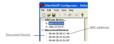
Like all Opto 22 Ethernet-based controllers and brains, each of the discovered devices has a unique hardware Media Access Control (MAC) address, which is displayed in the device list.
