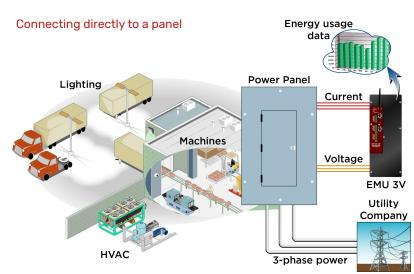
The Sensor can monitor energy devices in all ways, simultaneously:
