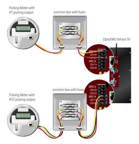
Use with either two-wire KY (Form A) or three-wire KYZ (Form C) pulsing devices.
