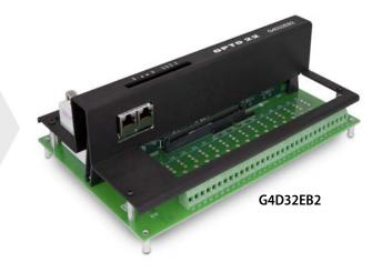
The G4D32EB2 is for new applications. For example, if you have a design that includes a G4D32RS, you could use the G4D32EB2 instead. It has the same footprint as the G4D32RS and the same field wiring.
