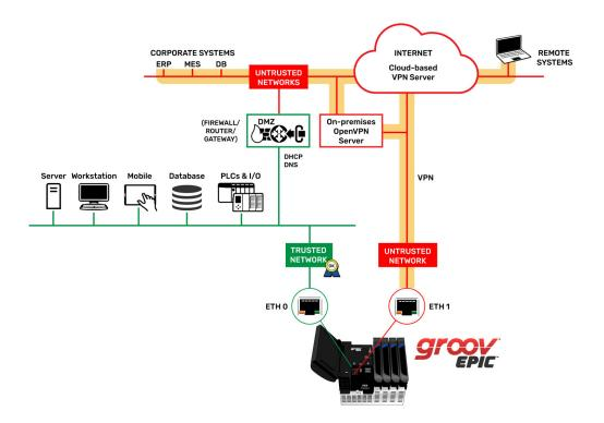
You can use *groov* Manage to configure VPN clients as additional network interfaces on your *groov* RIO or EPIC. These additional client interfaces connect to externally configured OpenVPN-compatible servers, allowing other clients connected to the same VPN server to access your *groov* product's software applications. OpenVPN servers can be located on premises, or in the cloud with VPN-as-a-service products like OpenVPN Cloud.
