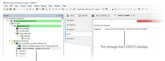
A GRV-R7-MM1001-10 with an unsupported combination of signal types on channels 0 & 1.
