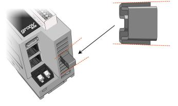
Thread a zip tie (not included) through the mount. Collect the wires into a bundle, wrap the zip tie around the bundle, then clip the excess zip tie.
