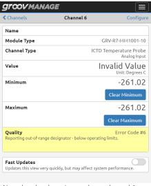
Note that the above image shows channel 6 configured to sense from an ICTD temperature probe. However, an actual probe has not been wired to channel 6 on this RIO, which means that RIO is sensing values that are out of range from this configuration. RIO reports this as a quality error.
