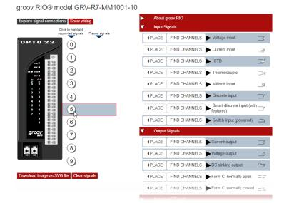
To see which channels can be configured with a specific function and signal, find the function and signal in the lists at right. Click the FIND CHANNELS button, and the Explorer highlights the channels that support that combination.
