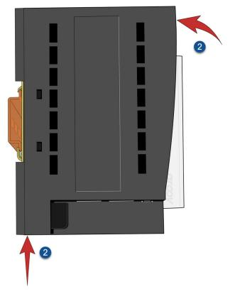
Before you release RIO, verify that the top and bottom of the DIN rail adapters have engaged the DIN rail.
