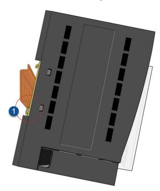
2. Push the bottom part of RIO upward, making sure that you feel the clip catch on to the rail, and simultaneously push the top half of RIO toward the DIN rail until the top of the DIN rail adapter engages the top lip of the DIN rail.
