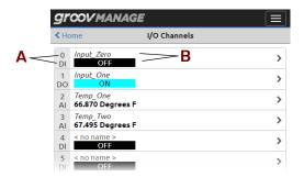
A The gray box shows the channel number at the top, the function and signal type on the bottom.
