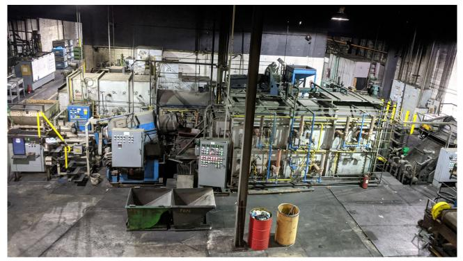
One of the upgraded furnace lines showing the new HMI at far left
